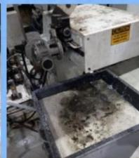
The Chip Collection Trolley where the Vacuum Cup is placed
