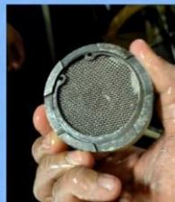
The Stainless Steel Vacuum Cup with Filter that sucks the coolant from the Chips Trolley
