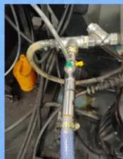
The Venturi Tube part of the Coolant Reclaimer is connected to the pump with a 'Tee'
